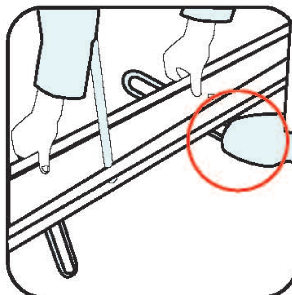
3. Retract the banner with both hands. Lock the print at the base.
